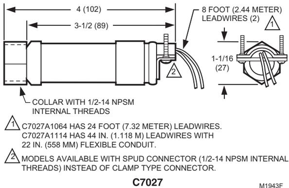
Fig. 1. Installation dimensions of C7027A in in. (mm).
